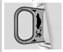
This handle will glow following exposure to light. Pull the release handle to open the hatch/boot from the inside.
