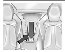
As passenger compartment trims require removal to access the fuse box, it is recommended this is performed by a dealer.
