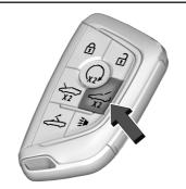
Press x2 on the remote key two times quickly. See Remote Keyless Entry (RKE)
