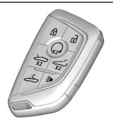
☐: Press to lock both doors and the fuel door. The turn signal indicators may flash and/or the horn may sound on the second press to indicate locking. See "Remote Lock, Unlock, Start" under Vehicle Personalisation ⇒ 82.
