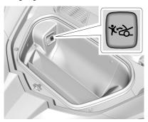
The under-bonnet compartment is equipped with a glow-in-the-dark emergency bonnet release button. This button will glow following exposure to light. Press the button to open the bonnet from inside the under-bonnet compartment.
