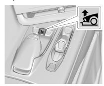
To use the front lift system, press the button on the centre console to raise or lower the vehicle. This feature can be operated at speeds up to 38 km/h when the
