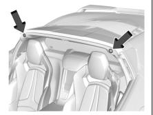
5. Position the rear edge of the roof panel next to the weatherstrip on the back of the roof opening. Then align and fit the pins at the rear of the roof panel inside the openings in the rear overhead weatherstrip. Gently lower the front edge of the roof panel to the front of the roof opening.
