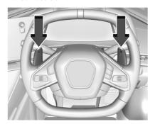
With the transmission in D (Drive), press the M (Manual Mode) switch on the centre console to enter Manual Mode. Use the paddles on the steering wheel to manually
