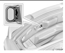
There is a glow-in-the-dark emergency hatch/boot release handle on the inside back wall of the storage compartment.
