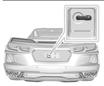
Remove the number plate to access the backup key lock cylinder for the boot. Insert the key and turn 90°.
