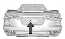
Use the mechanical key in the backup key cylinder behind the licence plate to manually open the hatch/boot. The licence plate must be removed.
