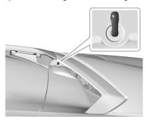
In the air inlet located on the body, rearward of the left door handle. Insert the key and turn 90°.
