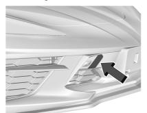
Carefully open the cover that conceals the front tow eye socket by using the small notch on the lower edge.
