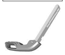
The mechanical key can be used to open the vehicle and hatch/boot if power to the vehicle is lost. See *Hatch* (Boot)  $\Rightarrow$  20.
