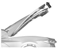
To provide more access to the engine or boot areas, the hatch/boot can be manually pushed up for additional travel. Do not apply excessive force.
