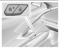
The passenger power door lock switch can also be used to lock or unlock the doors.
