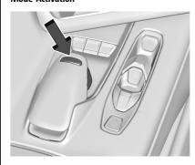
To activate My Mode, Weather, Tour, Sport and Track Mode, turn the Driver Mode Control (DMC) knob on the centre console to make a mode selection. When a mode is selected, an indicator will come on in the instrument cluster and stay on.
