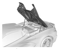
5. Hold 📤 until the tonneau cover is completely opened. The turn signals will flash once.
